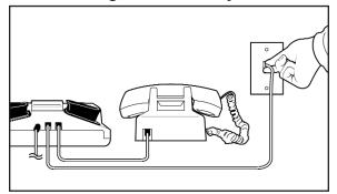
Plug one end of your modular into the telephone wall jack. Plug the other end into either jack on the back of your TDD. The second jack can be used to connect your telephone set or signaling device to the TDD.
