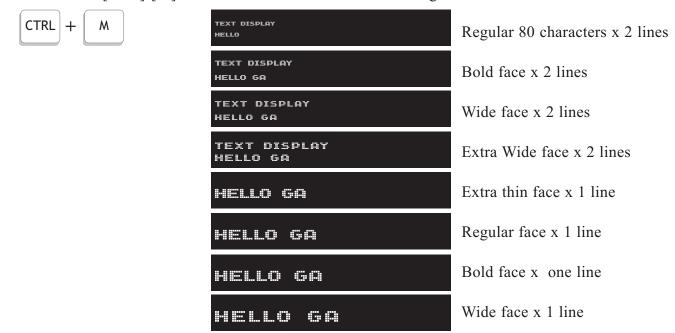
The TDD will print out the sign on message to check the font size, continue to press [CTRL]-[M] until you reach the desired font.
