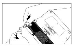
It is suggested that you exercise the battery in your Krown 200 at least once a month. That is, operate the unit on battery power until it needs recharging. Then recharge the battery by plugging in the AC charger/adapter for 12 to 14 hours. (The unit must be turned OFF in order to recharge.) Repeat this cycle at least once a month. When used regularly in this cycle, the battery should last for about three years.
