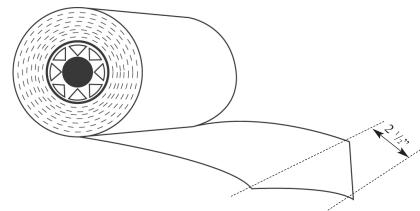
Place the paper roll spindle that you removed in Step 1 into the hole in the center of the paper roll.
