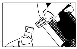
The replaceable, sealed battery pack is a single unit that contains the battery, connector and cover. This unit is located on the underside of the Krown 200 at the back of the unit. Replacement battery packs are available from Krown Manufacturing or your local Krown distributor.
