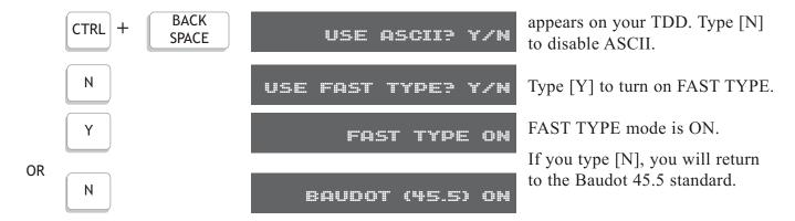
Note: If you select FAST TYPE ON, your TDD will still automatically communicate with older TDDs or with TDDs that do not have FAST TYPE in BAUDOT TDD Code (45.5 Baud).
