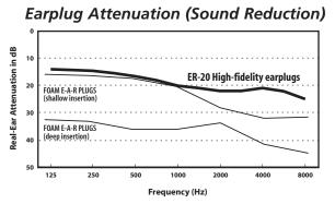
The above graph shows that ER-20s provide almost equal sound reduction (20 dB) across the range of hearing. Foam earplugs muffle the high frequencies of speech and music.
