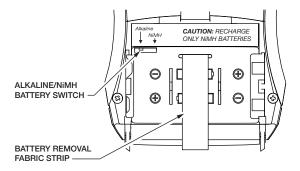
IMPORTANT: If non-rechargeable batteries are being installed, slide the battery selection switch in the battery compartment to the "alkaline" position. See Figure L below. If installing NiMH (or rechargeable) batteries, slide the battery selection switch to the "NiMH" position.
