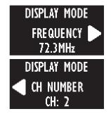
4. 8-channel mode restricts the transmitter to just the 8 non-interfering (simulataneous broadcast) channels. To change the transmitter between 8-channel and 17-channel modes, push the menu button until you see the channel selection mode screen, below. Use the arrow buttons to toggle between "17 CHANNEL MODE" or "8 CHANNEL MODE".
