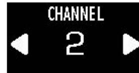
Push either arrow button to **step** to one of the 17 channels (above) -or- push-and-hold either arrow button to **seek** to the next active channel (below). The receiver is seeking the next *frequency*, so channels may appear out of order when seeking.
