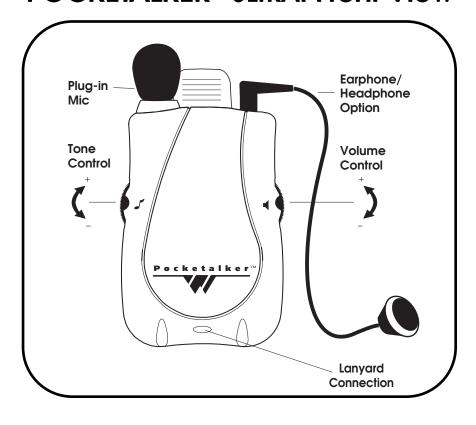
6. Turn on the POCKETALKER® ULTRA by turning the Volume Control counter-clockwise. The red "on" indicator light on the top of the unit should be lit.
