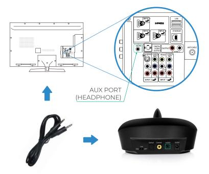
Plug one end of the AUX cable into the TV's AUX Port. Plug the other end into the AUX Port on the back of the transmitter. No sound will come through the TV if using AUX. Sound will only come through the headphones. Adjust the volume of your TV if you cannot hear anything coming from the Headphones.
