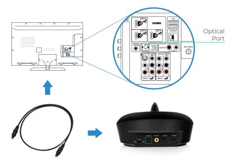
This method allows sound to be heard through the headphones and the TV. If you need sound to come only through the headphones, mute the TV. This jack may be called Toslink, Optical, or Digital Audio Output. Plug one head of the provided optical cable into this jack on your TV, while the other head into the Optical input on the back of the transmitter base.
