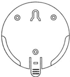
The Hanging wall tray can use double-sided adhesive or screw installed in the metope of smooth surface or cabinets lining, And also can be used flat on the table, More humane.
