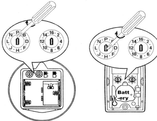
A transmitter and a receiver Coding turntable keep to work in the same direction, For example, transmitter turntable for "P" and "16", Receiver turntable for "P" and "16", too, If you find a neighbor's use with the same product, you can choose another code to prevent interference. Working mode can choose lighth or flash, Time can be set for 15 sec or 90 sec.
