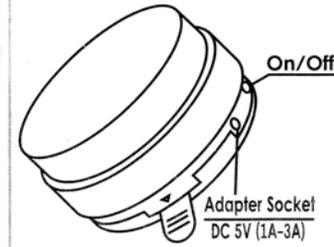
Product has a independent switch button, Press the button can be directly used as a flashlight. When the received signal lighting or flashing, Press the button to turn off led directly, Easy to use.
