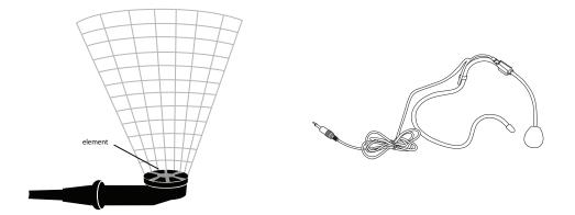
The LA-278 has a uni-directional pickup pattern. This means that the microphone's element must be oriented towards your mouth. It will not pick up audio very well from the side of the microphone. The main advantage of this type of microphone is that it helps minimize feedback and picks up less environmental noise.
