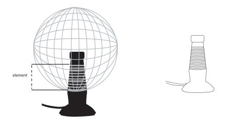
The LA-277 has an omni-directional pickup pattern. This means that audio from a broader area can be picked up by the microphone element. The main advantage of this type of microphone is that it does not have to be oriented directly towards your mouth for good audio pickup.
