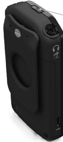
To view the unit ID, battery status or channel while the unit is powered, momentarily press the power button. To turn the receiver off, press and hold the power button for 3 seconds.
