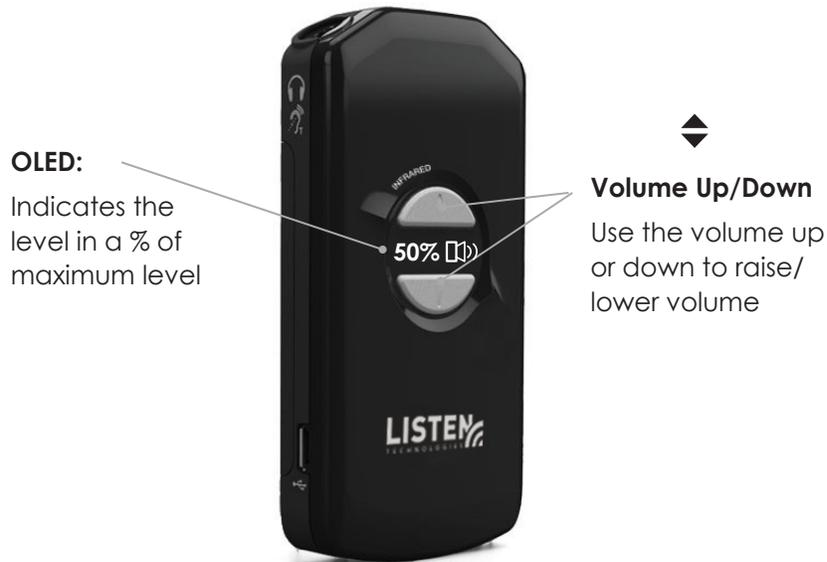
If the volume is adjusted while there is no audio present the unit will output a momentary tone each time the button is pressed allowing the user to gauge and adjust the audio level to a comfortable listening level. The volume level will be displayed for 3 seconds and then the display will turn off.
