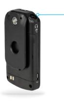
**Status LED:** Begins to flash when receiver has less than an estimated 3 hours use left on the charge.
