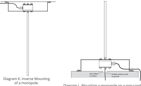
Diagram L. Mounting a monopole on a non-conductive surface. Use of the flexible wire creates a dipole, which is a better antenna than the monopole.
