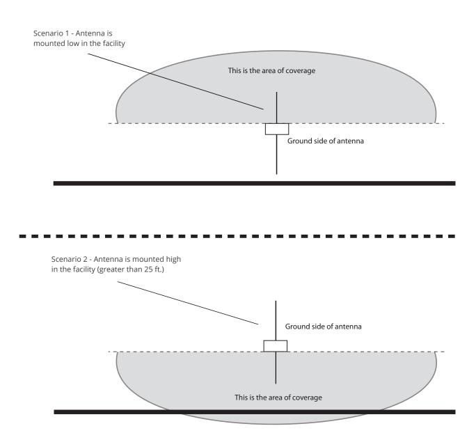
Diagram A. Antenna coverage patterns. In Scenario 1, the antenna is mounted low in the facility. The GROUND side of the antenna (marked on the module) should face down. In Scenario 2, the antenna is mounted high in the facility. The GROUND side of the antenna should face up.
