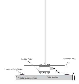
Diagram J. A reversed Antenna Module with Ground Plane and Shorting Plate.
