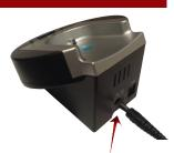
Plug AC Adapter into the base and into a power outlet.
