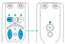
The sound from the Transmitter Unit is mixed with the sound from the internal microphone. You can adjust the balance between the Receiver Unit and the Transmitter Unit's microphone by holding down the M button(5) at the same time as setting the balance using the < (11) or > buttons (12).
