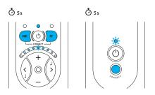
A "running light" on the Receiver Unit's Volume and Tone LED Indicator (8) moving towards the centre indicates that the link has been established.
