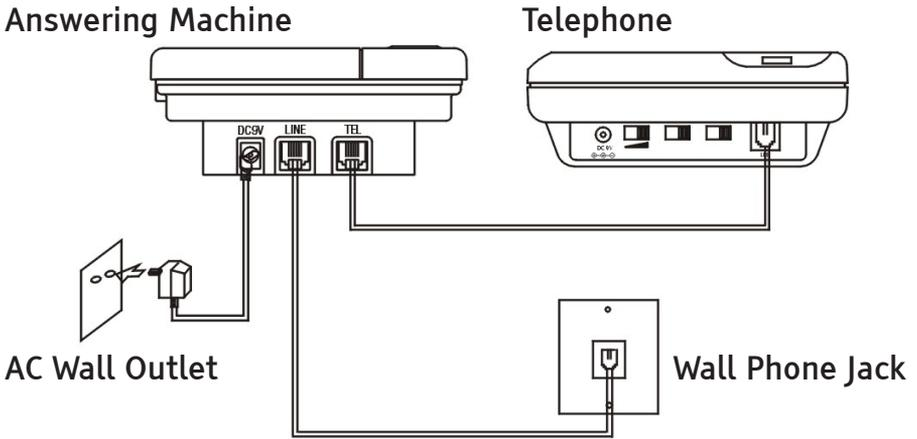
1. Connect one end of the telephone cord to the LINE jack on the back of the ANS3000 and connect the other end to a modular phone jack.
