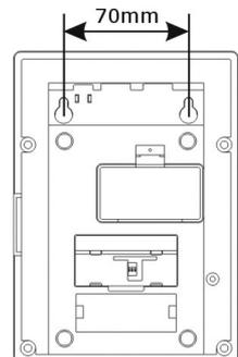
the mounting screws so they are hooked into the left and right keyhole slots. Slowly slide the unit down until it snaps into place.
