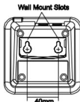
Place 2 screws into the wall then slots on the bottom of the base over the two screws heads and pull down to lock into place.
