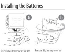
Remove lid / battery cover by two AAA batteries are packaged turning counterclockwise. in the small inner box. Remove the
