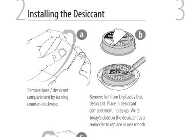
Re-attach the base to the drying unit by aligning tabs on the base with notches on the unit. Turn clockwise to close.
