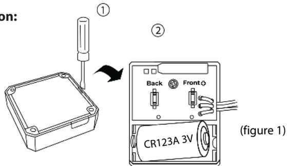
1. Open the front cover by insert a small flat-head screw driver (figure 1) into the small notch on the cover & gently pushing in.
