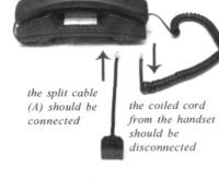
4) Attach the clip end of cable (1) in the free jack on the splitter cable (A) and the other end in the jack on the right side of the base unit.
