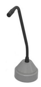
The M300 is a cardioid microphone that instinctively filters background noise, isolating the voice of the speaker. The weighted base and flexible gooseneck stem make the microphone ideal for counter, booth, or desk locations. The M300 is compatible with the counter loop systems and the Portable Info Loop (PIL).
