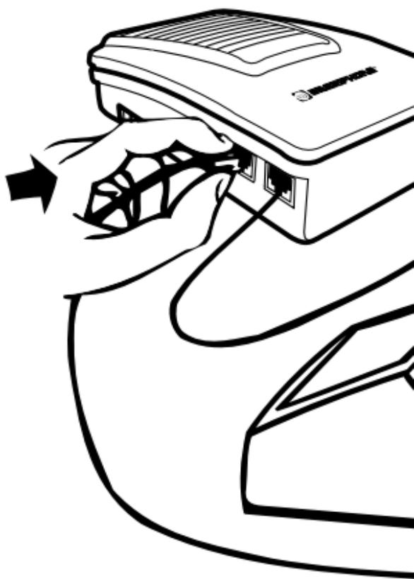
3. Connect one end of the cord provided with the unit into the PHONE jack of the Super Phone Ringer and the other end into your telephone.
