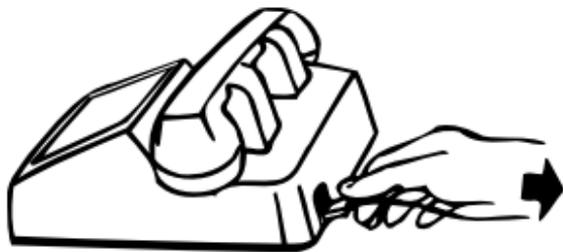
2. Plug the telephone line into the LINE jack of the Super Phone Ringer.
