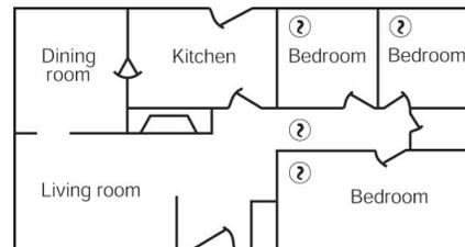
FIGURE 3: A SMOKE ALARM MUST BE LOCATED BETWEEN THE SLEEPING AREA AND THE REST OF THE DWELLING UNIT AS WELL AS IN EACH BEDROOM.
