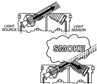
Under normal conditions, the light generated by the pulsing infrared LED is not seen by the light sensor, as it is positioned out of the direct path of the light beam. When smoke enters the sensing chamber, light from the pulsing LED light source is reflected by the smoke particles onto the photodiode light sensor. At the first sighting of smoke, the device is put into a pre-alarm mode. This is indicated by a rapidly flashing red LED on the face of the smoke/CO alarm.
