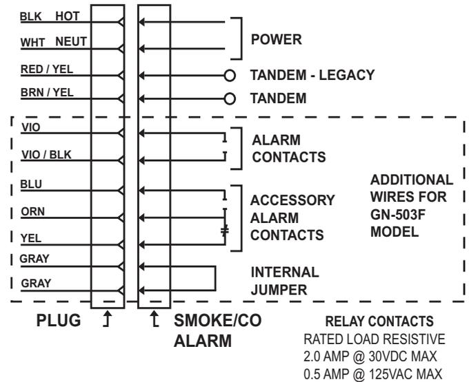
**CAUTION:** RED/YELLOW and BROWN/YELLOW wire to be capped when not in use. This wire is for tandem connection only. DO NOT connect to any other circuit.
