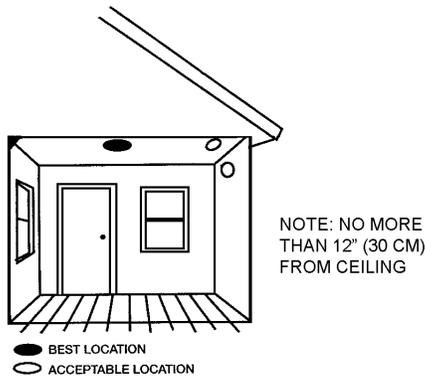
FIGURE 6: RECOMMENDED SMOKE/CO ALARM MOUNTING LOCATIONS
